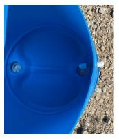
3. Cut a 3" length of ½" PVC pipe. Cut a 90degree elbow in half so you will have two pieces to glue on either end of the 3" PVC pipe, but just glue one side. Zip-tie some screening material on the glued end of the 3" piece of pipe; it is the first of two precautions to take to protect against mosquitos invading your soon-to-be-made water reservoir. Then, insert the tubing halfway into the overflow hole and glue the other elbow piece. The overflow pipe can be inserted from the inside
